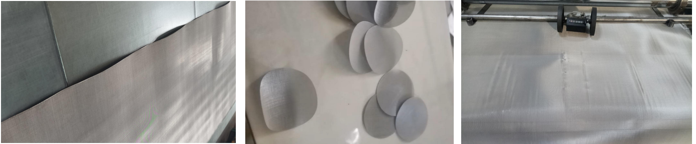
Gaps/ Wave edge/Not flat / Edged raised or edges curled after stamping / Defects or mechanical dama
