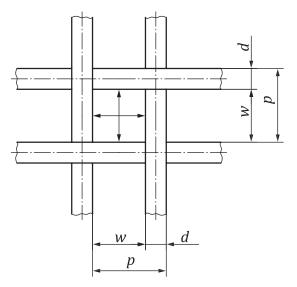
Figure 1 — Aperture width, wire diameter, and pitch
