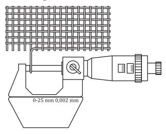
Figure 3 — Example of method for measuring wire diameters
