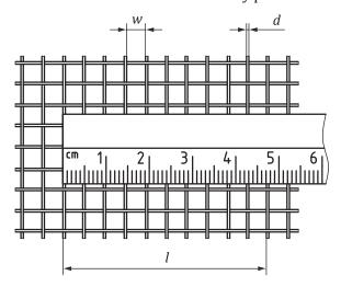
Figure 4 — Measured row with 10 pitches and 47,5 mm length
